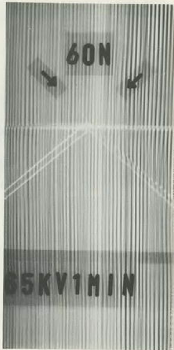
X-ray picture B The axial black lines display the grain of the wood. The horizontal lines and the mountain-shaped lines are the upper face of the male on the inside and the seam on the outside surface.
