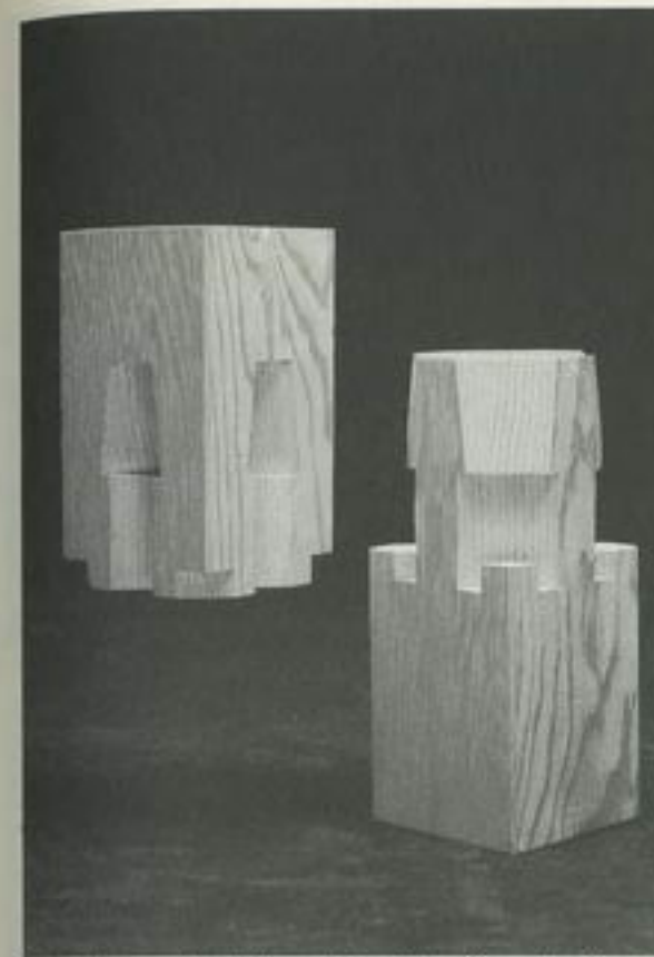
1 The male slides into the female diagonally.
