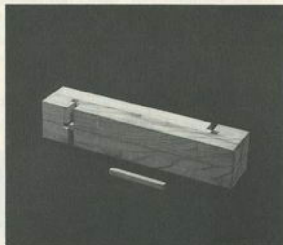
2 The surfaces of the middle drops (surfaces "d") touch
